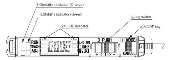
The SmartMark sensor sits on the front of the carriage of the Allen Datagraph Cutter or Digital Finishing System. It is the sensor that reads the presence or absence of a target that is printed on the media to allow the cutter to know where target is on the printed media.
