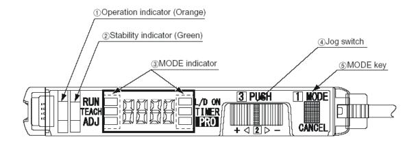
Normally you need to train the sensor every time you change either the media type, laminate type, or color of the target.
