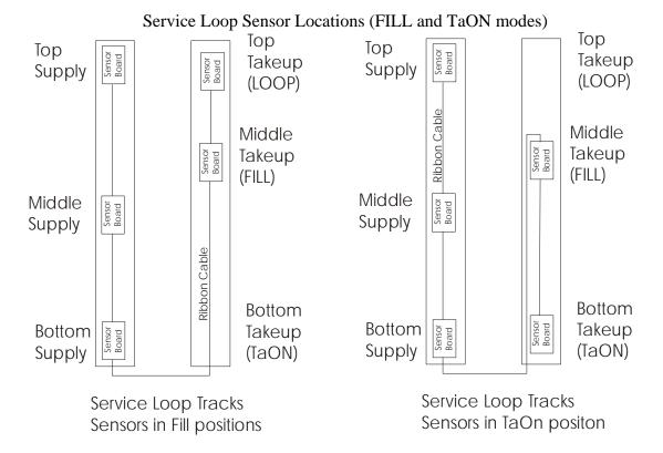
There are 5 sensors on DFS machines built after Dec 2004. The new machines are shipped with the last sensor on the ribbon cable installed in the top position on the take-up side.
