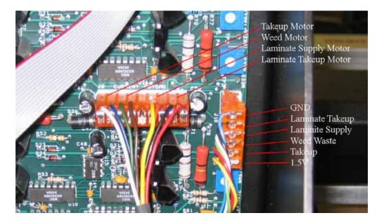
The photo above shows the mandrel motor connections and the mandrel pot connections to the control circuitry. J8 is routed to the reversing switches on the front panel and then to the motors. J10 is routed to the pots on the front panel
