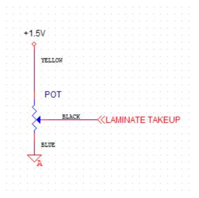
To determine if the problem is the control pot or the webamp board you can use a DVM set to DC volts with black wire connected to GND on connector (blue wire on photo) measure the voltage at pins 2, 3, 4 or 5 on J10. As you turn the associated pot on the front panel the voltage on the control pin should change between 0V and about 1.5V. If the voltage changes the problem is on the board. If the voltage does not change the problem is in the pot.
