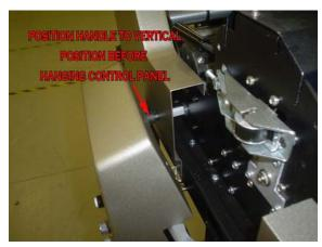
Step 3) Loosen the 3/8" locking nut on the Y axis belt tensioning assembly, then loosen the large, Phillips head y axis belt tensioning screw to relieve the tension on the y axis carriage belt.
