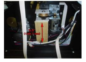
Step 9) Using the hammer and Phillips screwdriver, tap the shaft out of the bracket assembly. Inspect the shaft for any indentations from the setscrews. These should be removed prior to reassembly to aid with the installation of the shaft. Remove the large gold pulley and belt.
