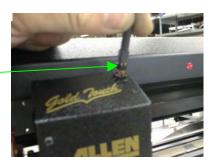
**Step 3-** Loosen set screw with the Allen wrench supplied in your accessory kit. Allow the tip to come into contact with the stainless steel platen. Use the Allen wrench to hold the red adapter at it's lowest position, with the tip still in contact with the stainless steel. Note the amount of element showing above the red adapter.
