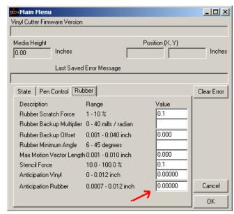
be concentric when cut on the rubber. The anticipation factor is set by visually inspecting resulting rubber cut and adjusting the anticipation factor to different values to make the plotted circle concentric.
