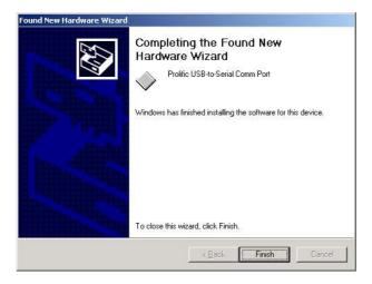
5.5.7 After the step, you have to check the "Control Panel"-"System""hardware"-"Device Manager" and you can see the (Prolific USB to Serial Comm Port) under the Ports (Com & LPT)
