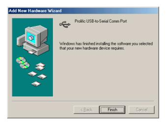
5.3.5 After install the driver, you have to check the "Control Panel""System"-"Device Manager" to make sure the driver has already installed, you can see a USB to Serial Port (COM3) under the Ports (COM & LPT) and a Prolific USB-to-serial Com Port under the Universal Serial Bus Controller.
