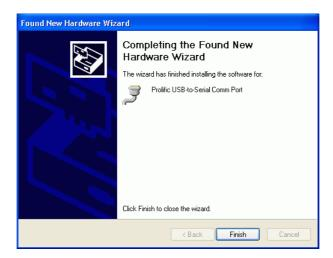
5.7.6 After install the driver, you can see a new **Prolific USB-to-Serial** Comm Port (COM3) under the Ports (COM&LPT).
