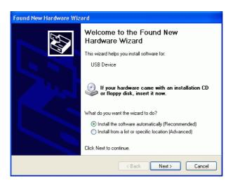
5.7.4 The windows will auto detect the device (prolific USB-to-Serial Comm Port) and install the driver into your system.
